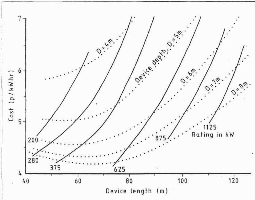
Figure 4 Estimated Cost of Electricity Produced by Small Scale SEA-Clams of Varying Dimensions.
