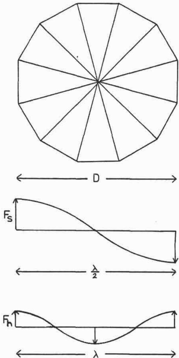
FIG. 10 WAVE PROFILES FOR MAXIMUM SURGE AND HEAVE LOADING
