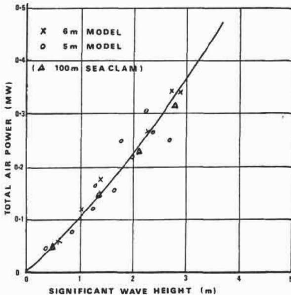
FIG. 9 SCALED AIR POWER RESULTS FOR 60 m DIAMETER CIRCULAR SEA CLAM
