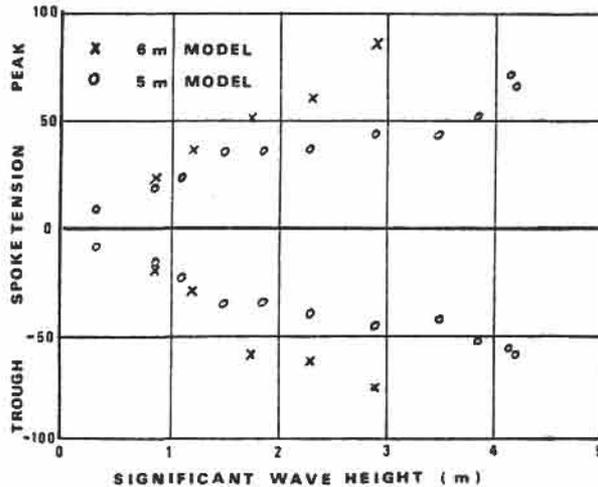
FIG. 11 SCALED SPOKE TENSION RESULTS FOR 60 m DIAMETER CIRCULAR SEA CLAM
