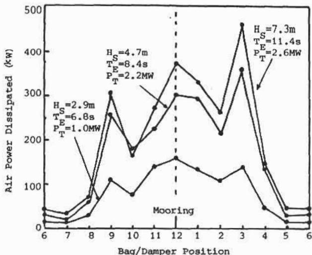
Fig.8. Scaled Air Power Distribution Around Circular SEA Clam
