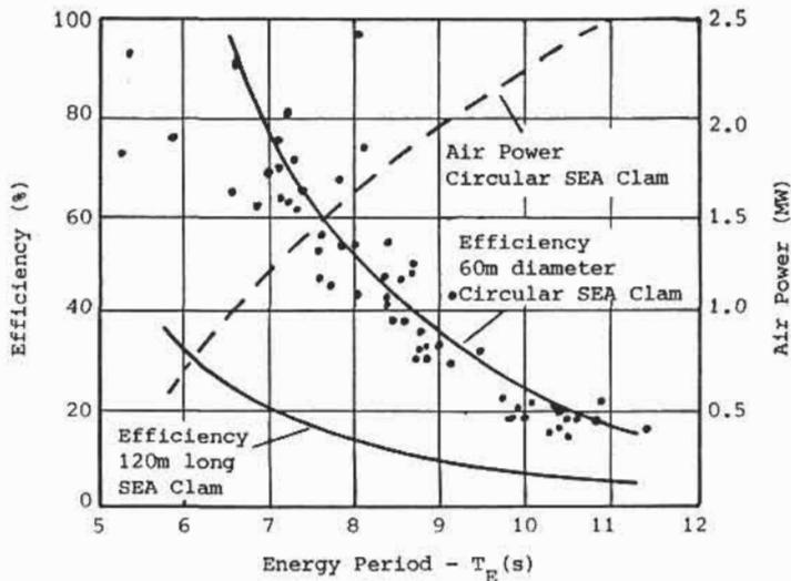
Fig.7. Scaled Air Power Results for 60 m Diameter Circular SEA Clam
