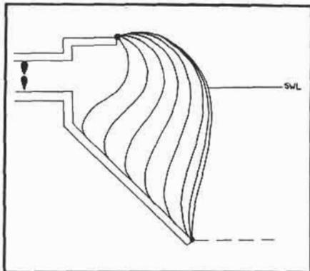
Fig. 5. A series of membrane profiles obtained by computing the shapes for a range of gauge pressures. All other parameters such as frame and saddle angles, depth of immersion, length of fabric are held constant.
