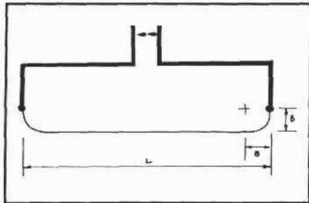
Fig. 4. A horizontal cross-section of a cell at the still water line
