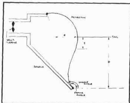
**Fig. 3. A schematic vertical cross-section of one air cell for the Clam**
