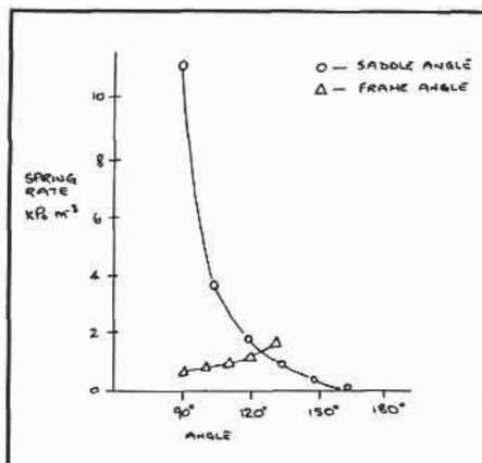
Fig. 6. The influence of saddle and frame angles on the cell spring rate
