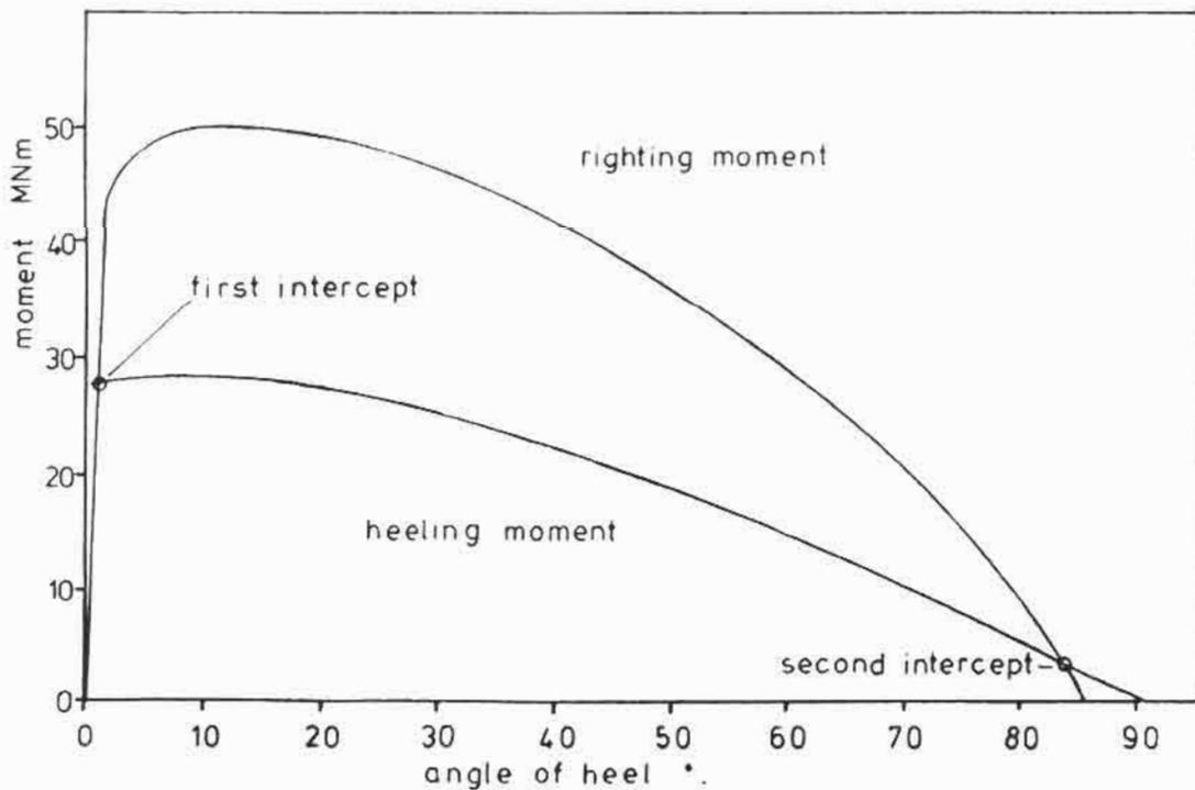
FIGURE 3.3 RIGHTING MOMENT FOR COMPARTMENT DAMAGE CASE.
