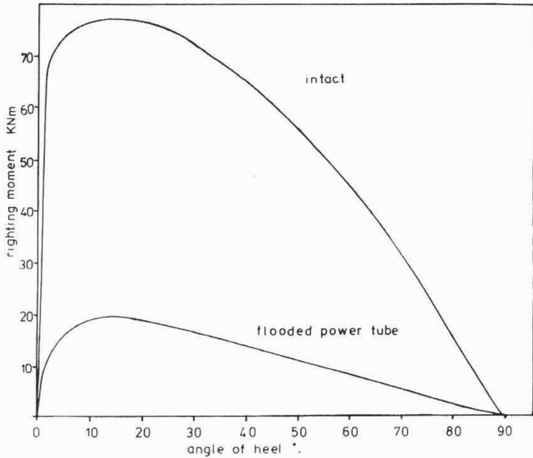
FIGURE 3.2 COMPARISON OF RIGHTING MOMENT CURVE FOR INTACT CASE AND FLOODED POWER TUBE CASE.
