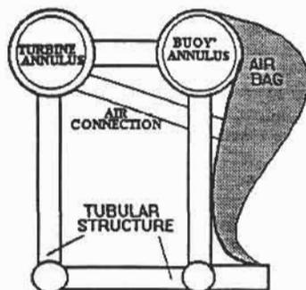
Fig. 2 Tubular Steel Design - 1986
