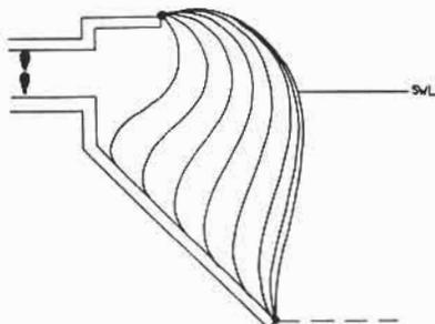
Fig. 4. A series of membrane profiles obtained by computing the shapes for a range of gauge pressures
