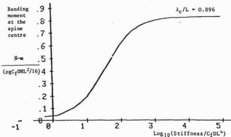
FIGURE 1 BENDING MOMENT-STIFFNESS UNIVERSAL CURVE
