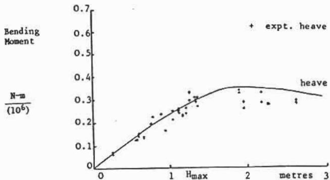
FIGURE 8 BENDING MOMENT v  $H_{max}$
