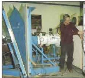
Bag-turbine-alternator rig under test at Coventry Lanchester Polytechnic.
