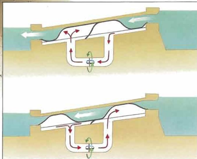
air flow through the turbine which can be used to drive a generator at synchronous speed. Output power control is achieved by varying the volume of air in the system.
