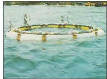
Circular SEA Clam wave energy model on test on Loch Ness.
