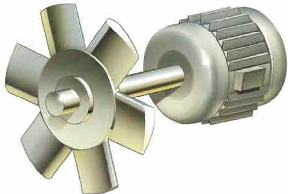
Wells type rotor directly coupled to electrical generator.
