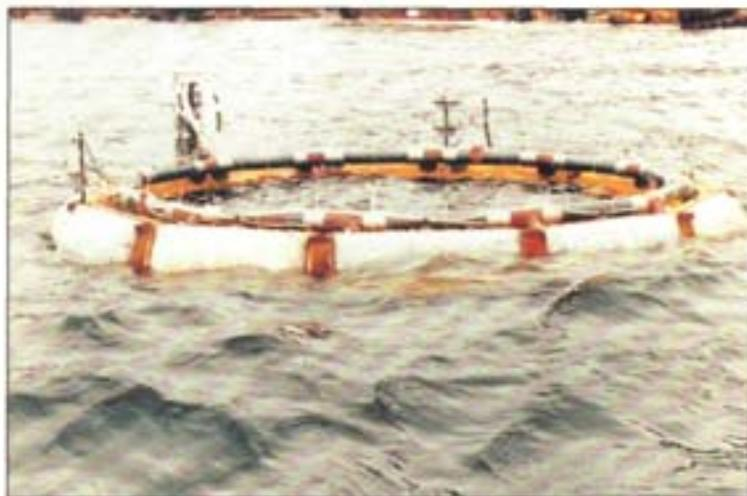
The SEA Clam wave energy converter - model under test on Loch Ness
